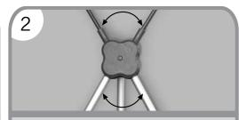
2. Press the button in the center of the connector to unfold the rods to the width of the
